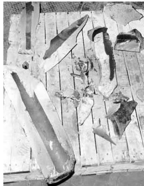
Figure D-3: Pieces of shattered press stem.
