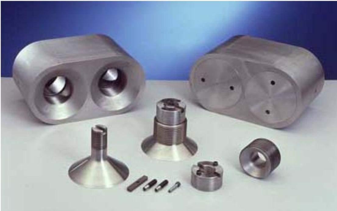
Figure 3-4: Fixed dummy block for oblong billet
