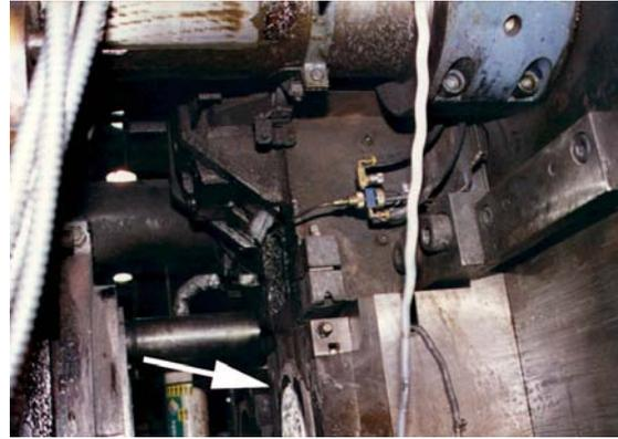
Figure 3-19: Proper lubrication of the butt shear results in a clean and complete removal of the butt from the die.
