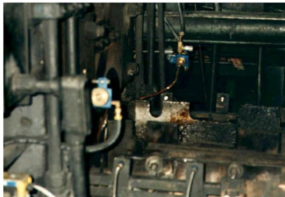
Figure 3-21: Remote mounting of nozzles away from the heat allows for easy adjustment and repair.
