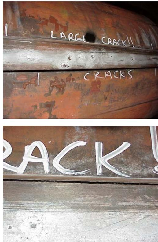
Figure 3-10: Container with crack through keyway, probably caused by overheating. A larger radius may help eliminate this problem
