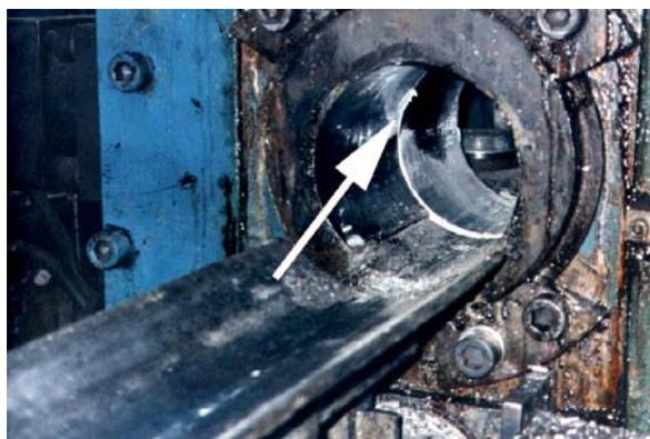
Figure 3-18: Left unlubricated, tools build up metal that eventually leads to problems.
