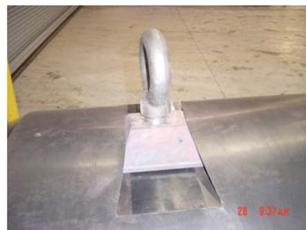
Figure 3-9: Alternative “dove tail” design for container lifting.
