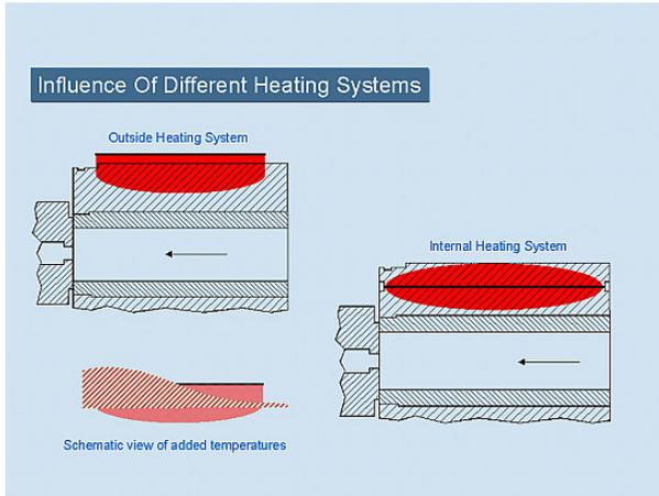
Figure 3-14: Influence of external vs. internal heating systems. (Illustration courtesy of Kind & Co.)
