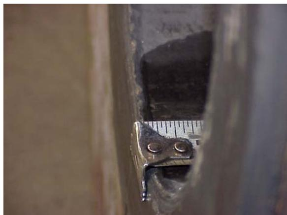
Figure 3-11: Liner with badly coined face, probably due to insufficient contact surface between die and liner face.
