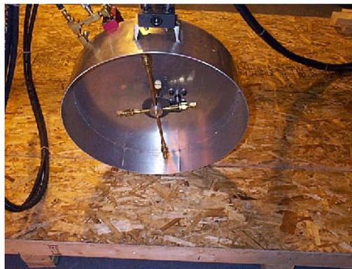
Figure 3-22: Rotating nozzles are driven with an air driven gearmotor for improved system reliability.
