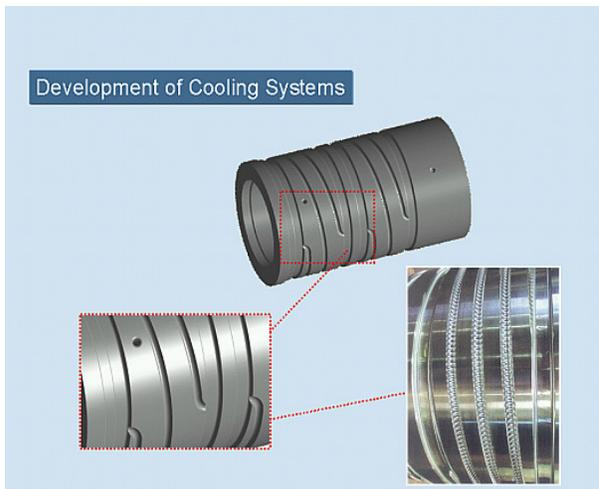
Figure 3-16: Container cooling grooves (Illustration courtesy of Kind & Co.)
