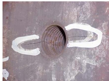
Figure 3-8: Container cracked through hole for lifting eye. Container was also overheated.
