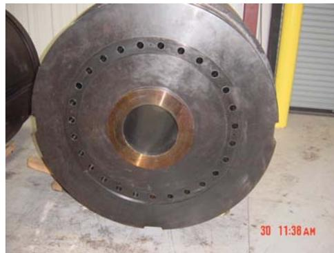
Figure 3-13: Container using heaters inserted into the mantle.
