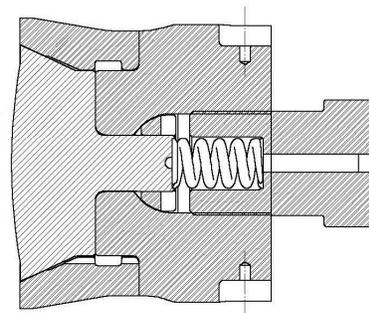
Figure 3-2: Fixed dummy block with replaceable wear ring
